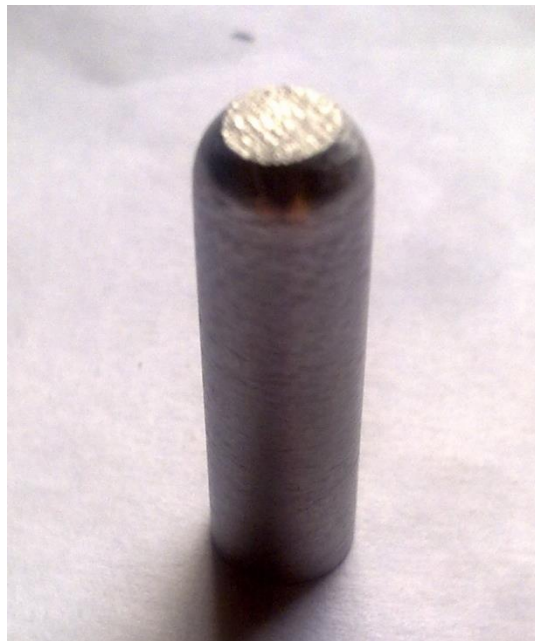
Fig. 5 Pin specimen made of AISI D3 steel (before wear)
