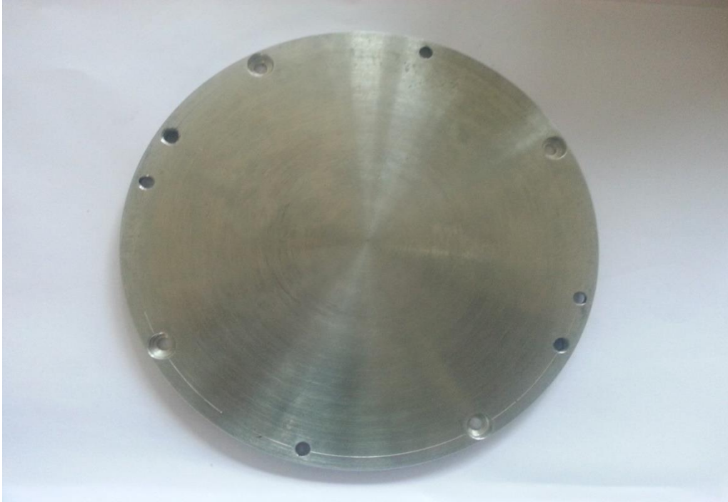
Fig. 8 AISI 1020 steel disk specimen (before wear)
