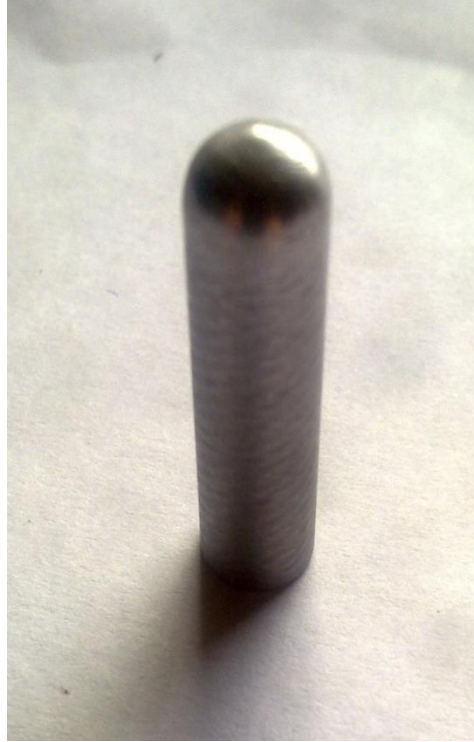
Fig. 5 Pin specimen made of AISI D3 steel (before wear)
